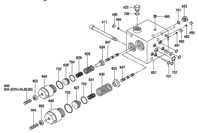
Torque Limit Module Detail
